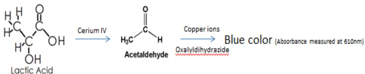
**Figure 3:** Principle of colorimetric estimation of lactic acid.
