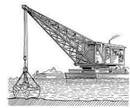
Dredging is the excavation of material from a water environment.
